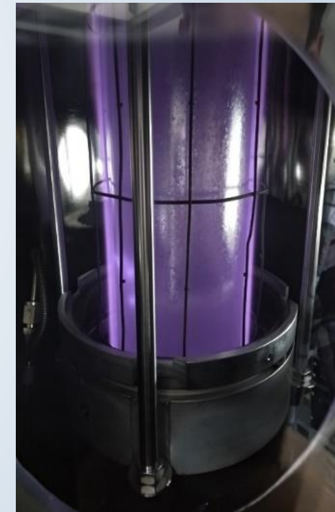
Nb cathode plasma cleaning
