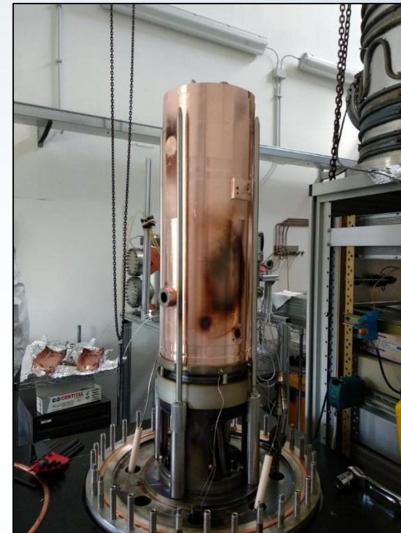
Cavity assembled on coating system
